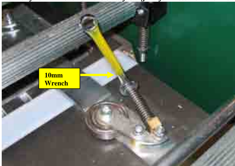
Picture of 10mm wrench on tension adjusting nut for Pressure Roller Bearing.
