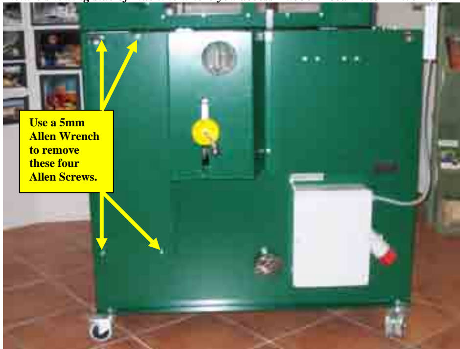
Picture showing side of machine where you access Rubber Feed Roller Drive Belt
